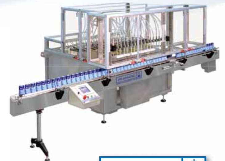
H-CE Molten Hot Filler Fills Products up to 200 Degrees Fahrenheit
