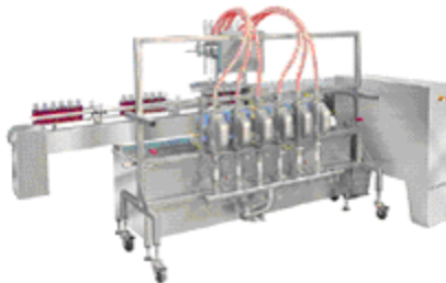
Fig. 2 Dockable Digifil™ Flowmeter Filling System (DFS) (Rear View)
