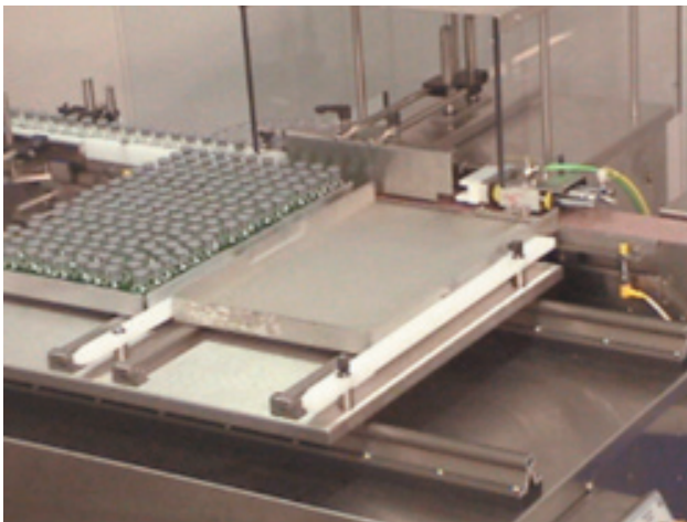
Shuttling Loading Deck
